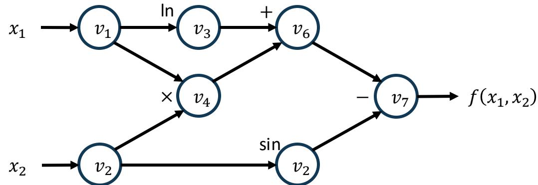
Each node represent an (intermediate) value in the computation. Edges present input output relations.
